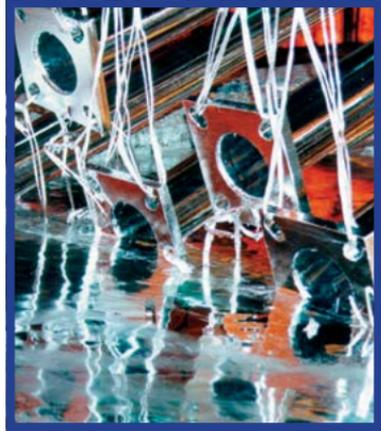
Whether bright or dull, the key factor in the newly galvanized condition is a lack of zinc compounds on the surface, which simplifies the cleaning. Some newly galvanized parts, those with a dull gray, can have a rough surface texture, while bright and shiny parts are often smooth. Regardless if the surface is rough or smooth, profiling the surface by sweep blasting is necessary to ensure the adherence of the paint system.
